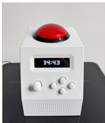
The finished unit. 140 by 160 by 170 mm, printed in two parts
