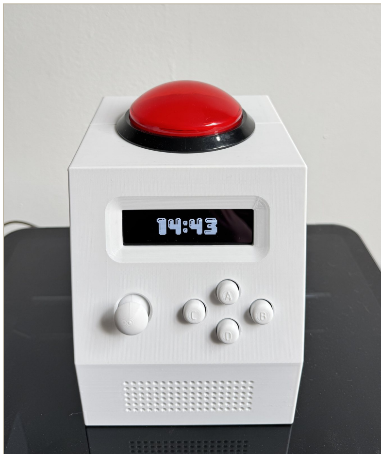
The finished unit. 140 by 160 by 170 mm, printed in two parts, with the 100 mm arcade button on top and the control face raked back 70 degrees for a bedside viewing angle.
